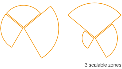
Detection zone for sensIQ S mounted at a height of 2.5 m black = tangential walking direction orange = radial walking direction
